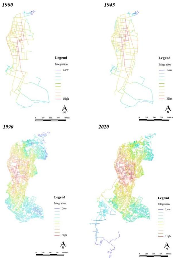
Figure 6. Global integration (Rad-N) analysis of Makassar city from 1900-2020 (based on axial models)
